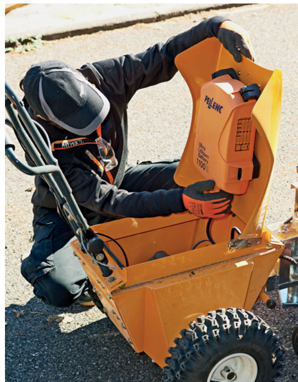
Easy access to the battery, protected in its housing
