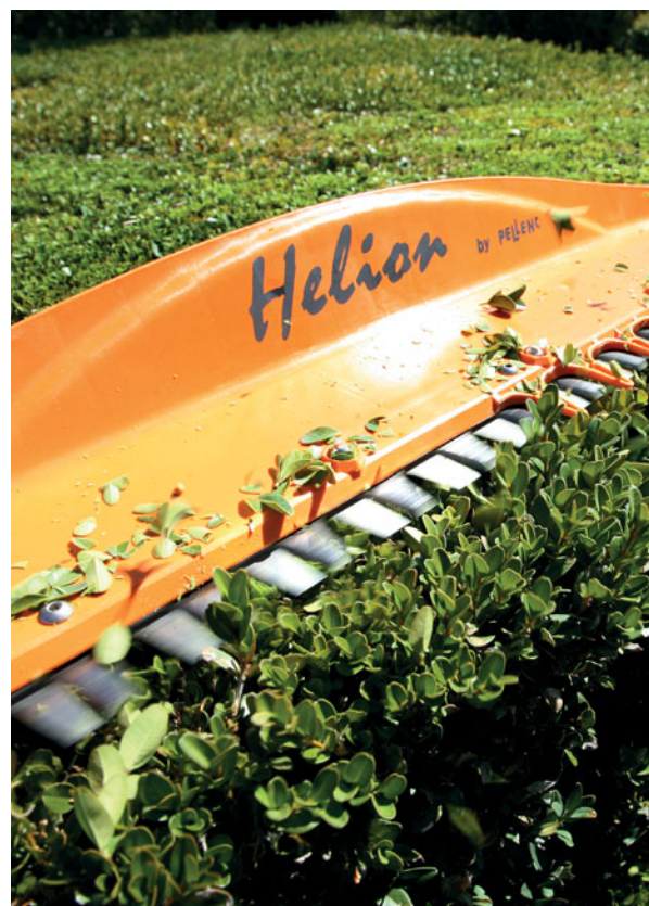
Adaptable deflector for the 63 cm cutter bar
