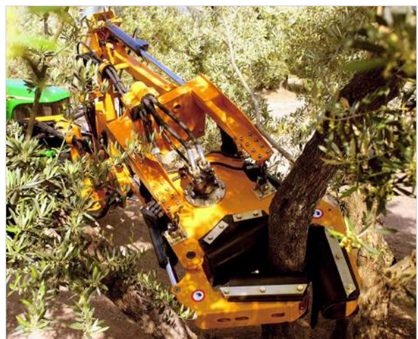
F100 with three-jaw pinch grip
