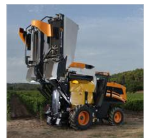
Bin emptying at 3 metres
