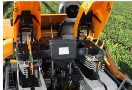
Synchronous drive destemmers
