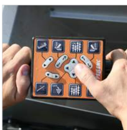
Remote control on the harvesting head.
