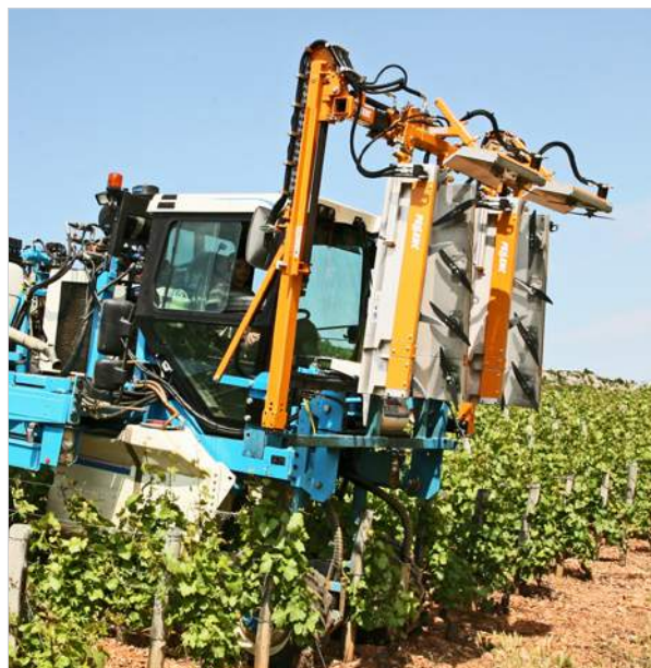
Vertical lifting of the trimmers
