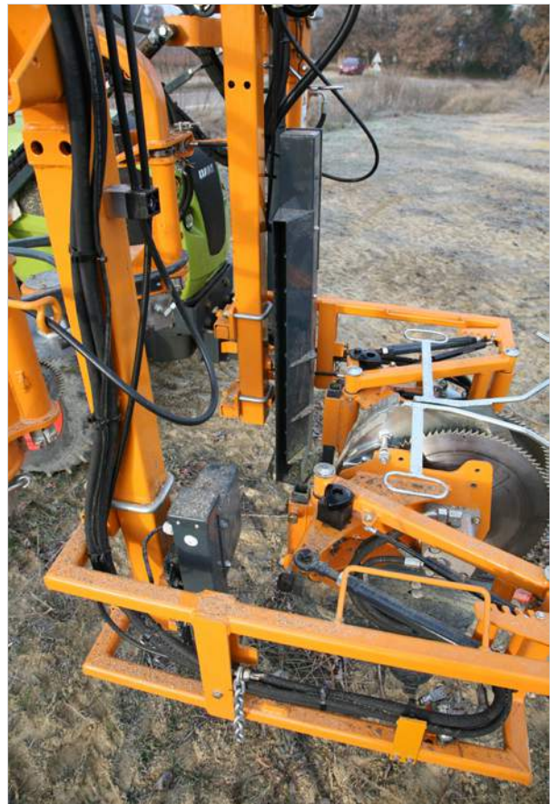
Automatic cordon tracker with the vision system.
