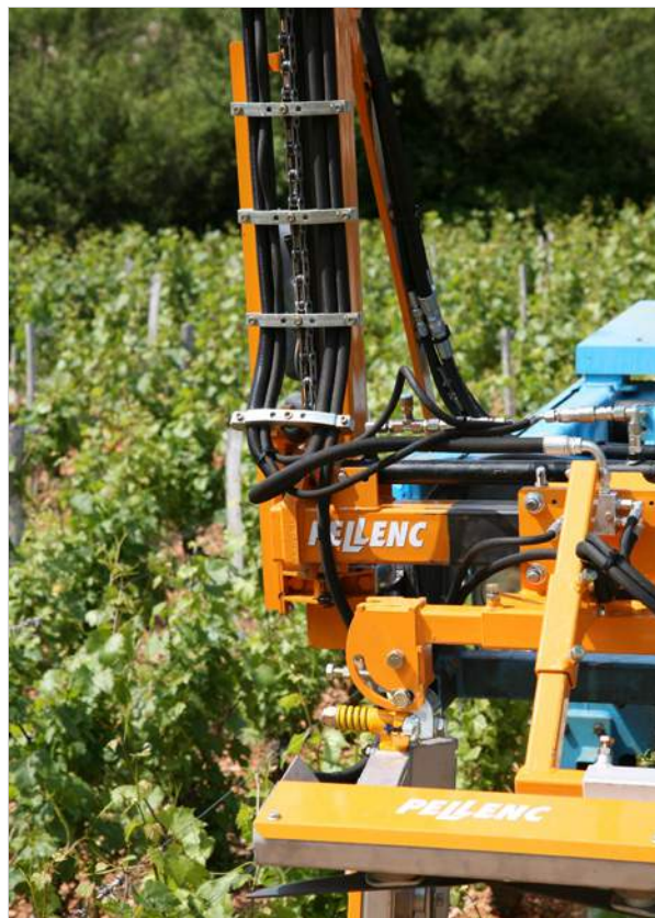
Guidance of the hoses by stainless steel chain
