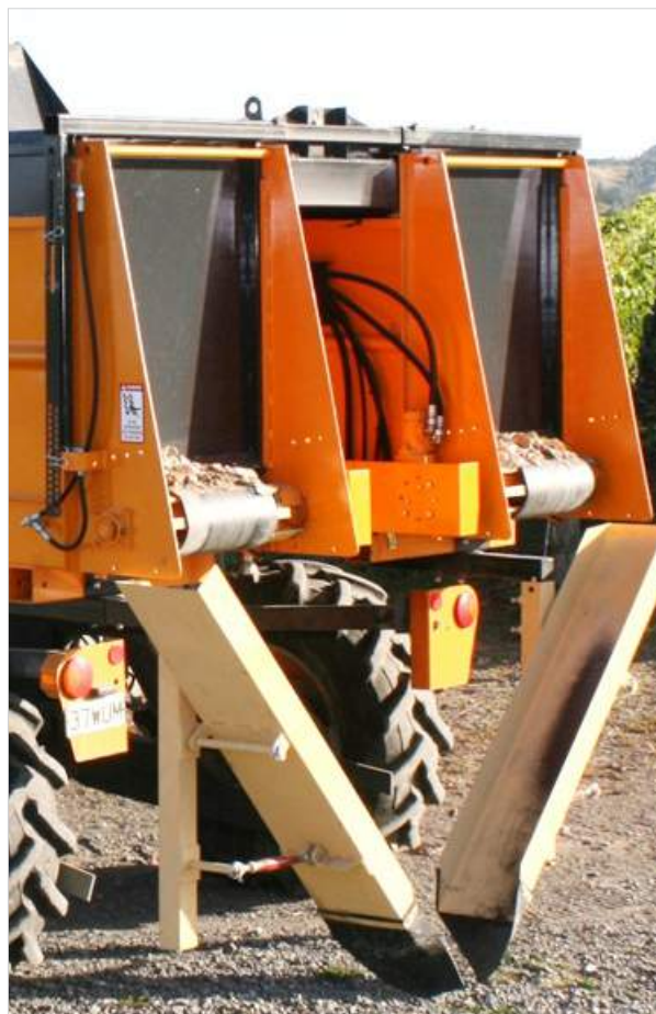
Spreading done at the base of the row
