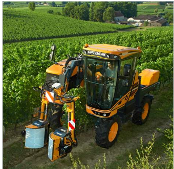
Full row leaf remover on the Optimum carrier
