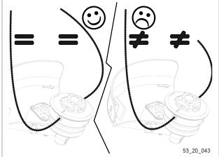
5. Turn the spool (23) clockwise to wind the strimmer wire.
