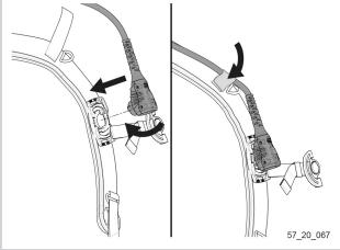
9. Connect the power cord (28) of the counterweight to the extension cord (29).
