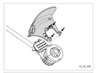
2. Tighten the 4 screws to a torque of 3.5 N.m using a T 25 screwdriver.
