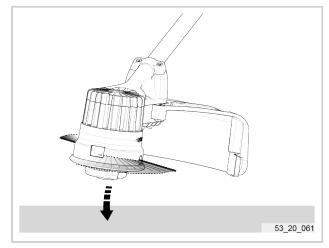
The cutting head plate in the protective guard automatically cuts the strimmer wire to the correct length.
