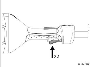
3. Keep the 2 triggers pressed for the tool to work.
