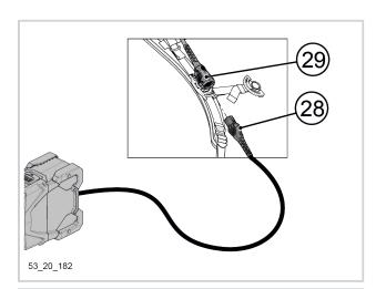
2. Turn the quick connector a quarter turn to remove the extension cord (29) from the shoulder strap or harness belt.
