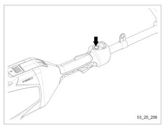
• Press one of the 2 on/off buttons on the battery.
