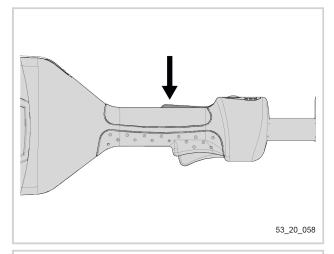
2. Press the control trigger twice to prime.
